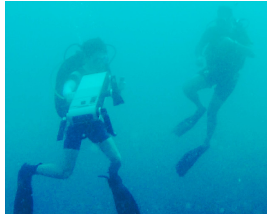
Fig. 1: Two divers collaborating with an underwater robot. It is desirable for the robot to be able to uniquely identify its human partners; however, the divers’ similar gear and the poor visibility conditions underwater make this difficult.
